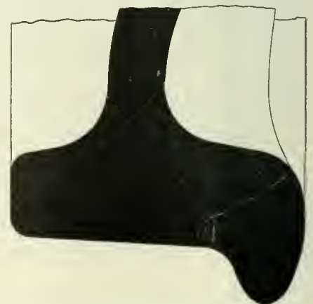
FIG. 3. CRACKS THROUGH FLANGE.
